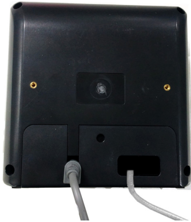
Figure 17: Cable installation completed
